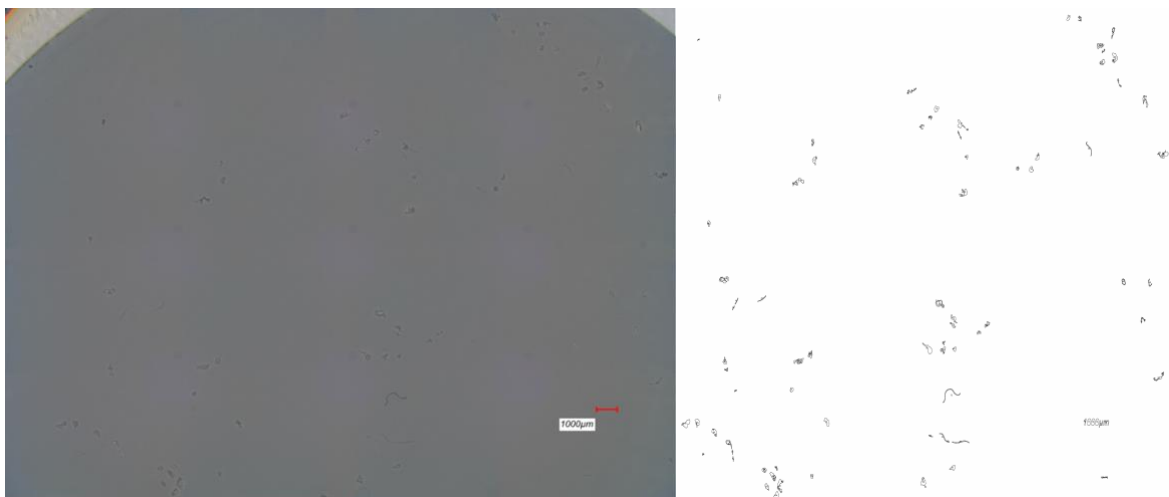
Figure 10: Left: Original microscope image, right: outline drawing of particles created with Fiji [73].
