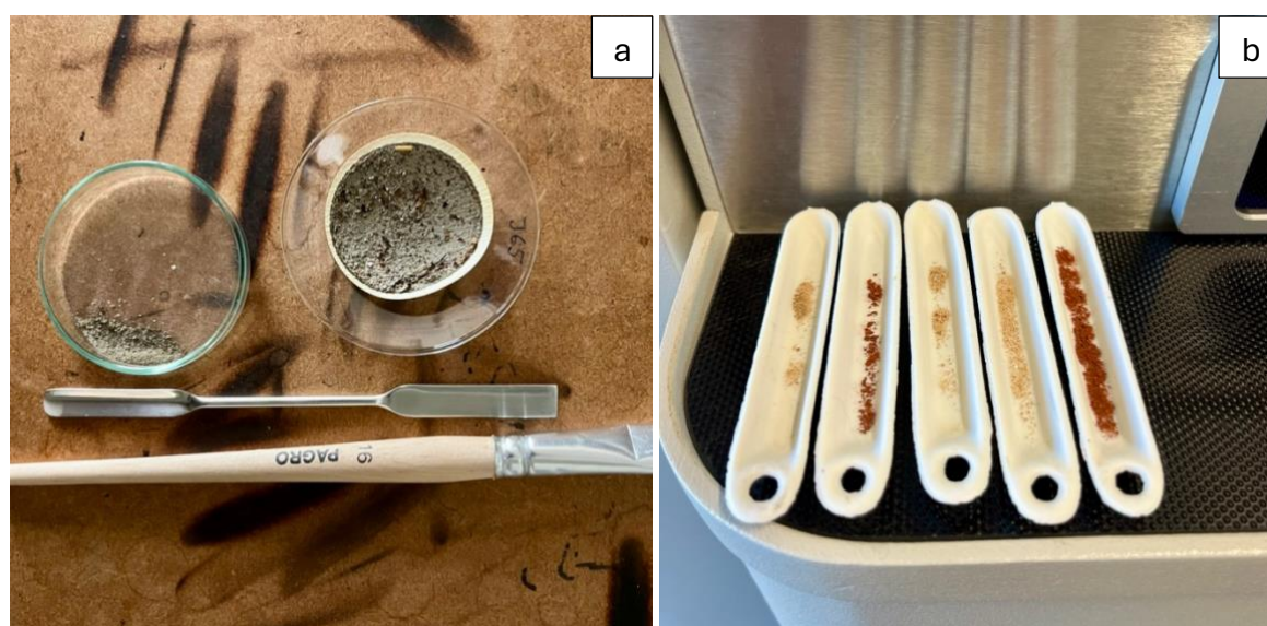
Figure 8: Measurement of TOC values. Fenton/compost residue preparation (a). Samples after combustion and TOC measurement, note: the reddish samples are from the maximum removal tests and clearly show the increased iron content (b).
