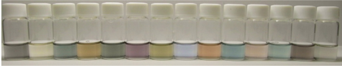
Figure 2.4: Colours of metallic and semiconducting SWCNTs with different diameters, graphic taken from [9].
