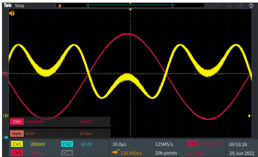
Figure 23: Signal output from the interferometer with 5m fiber.
