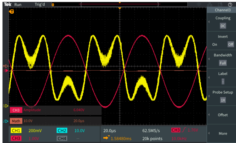
Figure 25: Signal output from the interferometer with 15m fiber.
