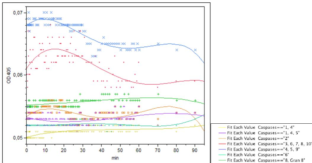
**Figure 4.16.** Plate reader results for first ground sample, OD at 405nm. Caspase activity measured using seven different substrates, each color represents one substrate. Corresponding caspases for each substrate shown in left box. Results still need to be normalized to a protein concentration of 1mg/ml.
