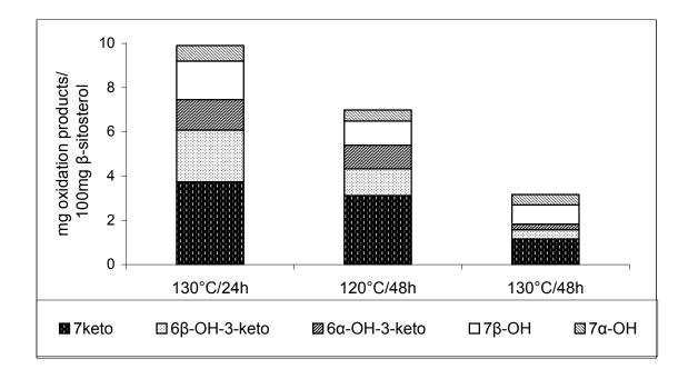
Fig 4.1 Proportion of collected  $\beta$ -sitosterol oxidation products (mg) after different oxidation conditions (130 °C/24 h, 120 °C/48 h and 130 °C/48 h) measured by GC-FID.
