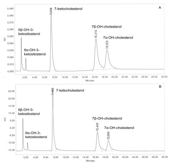
Fig 4.14 NP-HPLC chromatogram of cholesterol standards,  $6\beta$ -OH-3-ketositosterol and  $6\alpha$ -OH-3-ketositosterol with (A) UV detection at 206nm and (B) ELS-detection.
