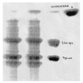
Fig 4.2 Oxidation products of  $\beta$ -sitosterol observed on silica TLC plates developed after spraying with 50% sulfuric acid and following heat treatment.
