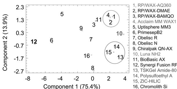
**Figure 13.** Results of the PCA on the HILIC-elution data: Score plot of the two first principal components.
