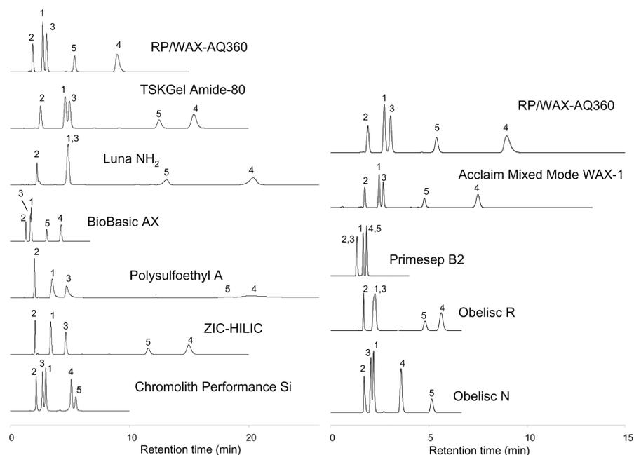
**Figure 11.** Chromatograms of the HILIC test for nucleosides. Experimental conditions see Section 2. Solutes: **1**, adenosine; **2**, thymidine; **3**, uridine; **4**, guanosine; **5**, cytidine. (Note, numbering corresponds to the elution order as expected from  $\log D$  values).
