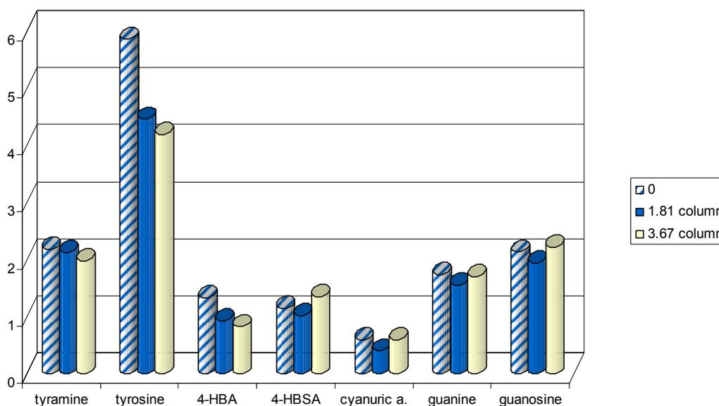
**Table 1** retention factors of different benzoic acid analogue on three columns. Mobile phase: ACN/100mM ammonium formate pH 7 (90/10)
