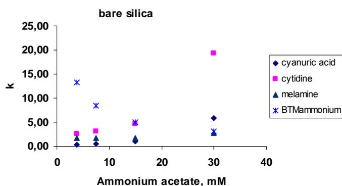
(6b) The effect of ammonium acetate concentration on retention factor on propylurea-bonded silica phase with ligand density  $3.67 \mu\text{mol.m}^{-2}$ .
