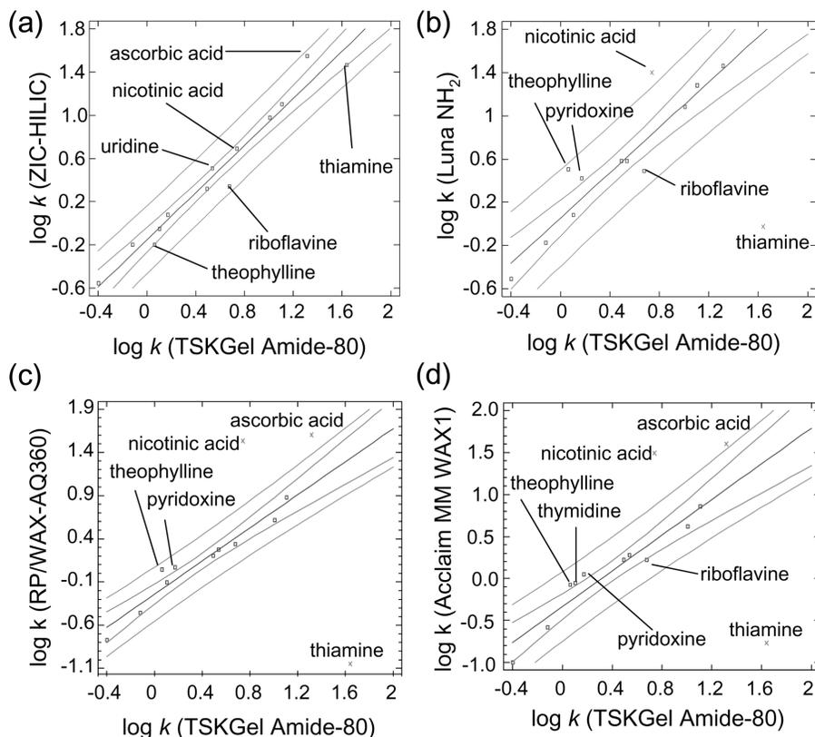
**Figure 12.** Orthogonality plots of  $\log k$  values from HILIC tests of TSKGel Amide-80 versus (a) ZIC-HILIC, (b) Luna NH<sub>2</sub>, (c) RP/WAX-AQ360, and (d) Acclaim Mixed-Mode WAX-1. Besides the fitted model the plots show the confidence (inner lines) and prediction limits (outer lines).
