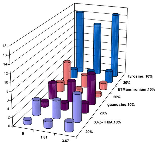
(5b) Illustration of response factor of retention for acidic, basic, neutral and zwitterionic solutes to the variation of water fraction in eluent from 10 to 20%.
