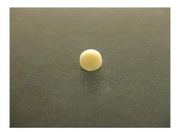
Figure 5.3: Pressed NaCl+Au-pellet.
