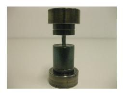
Figure 5.2: Mounted sample press.
