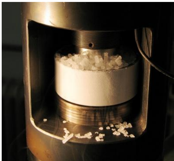
Figure 38. The anvil region of the HPT-facility at ESI Leoben, Austria, during operation at temperature of frozen CO 2 (195 K).
