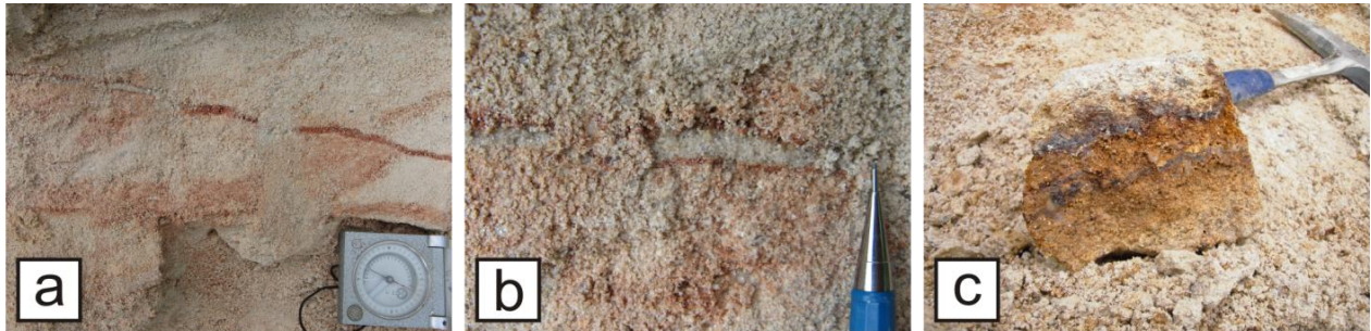
Fig. 28: Deformation bands in course grained conglomeratic sand ( a & b ) and sandstone block cemented by siderite/limonite ( c ), (outcrop CP_010, Lower Klikov Fm.).)
