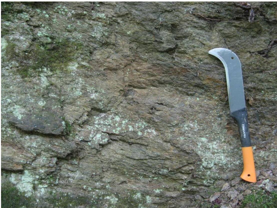
Fig. 15: Brittle fault zone in Bt-Ms-Paragneis with slightly W-dipping, sub-horizontal foliation (outcrop CP_001, Variscan, Moldanubian crystalline; viewing direction: SW).
