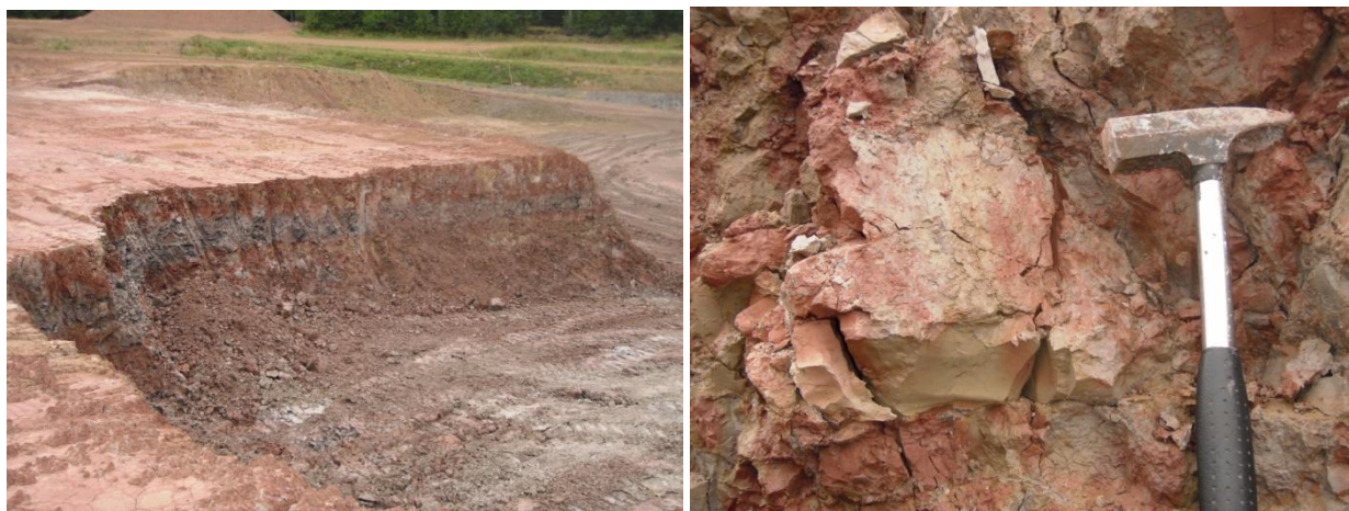
Fig. 8: Claypit north of Munice (Outcrop CP_002). The Reddish, greenish and grey claystones are typical for the top member (C) of the Klikov-Formation.
