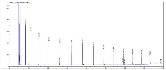
Figure 2: The chromatogram of the n-alcanes separated by the Supelcowax  $^{\rm TM}$  10 coloumn
