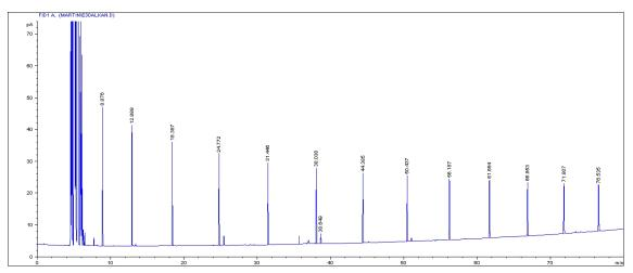
Figure 3 The chromatogram of the n-alcanes separated by the Equity™ - 1 coloumn
