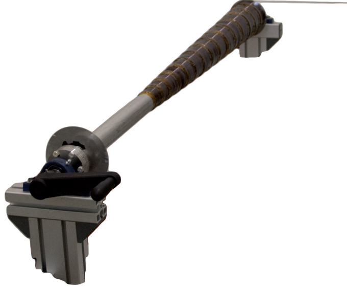
Figure 2.13: For building of the Zeeman slower the vacuum tube was mounted with ball bearings such that it can be rotated. A rectangular wire was carefully wound around the tube forming a tapered solenoid to create the required magnetic field to slow atoms inside the tube.
