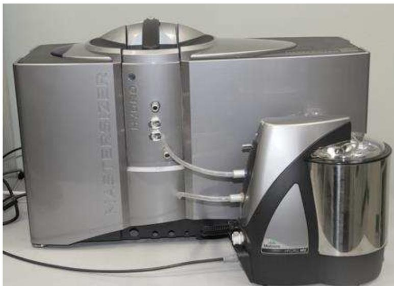
Abb. 14: Mastersizer 3000, Hydro MV, Malvern Instruments [43]
