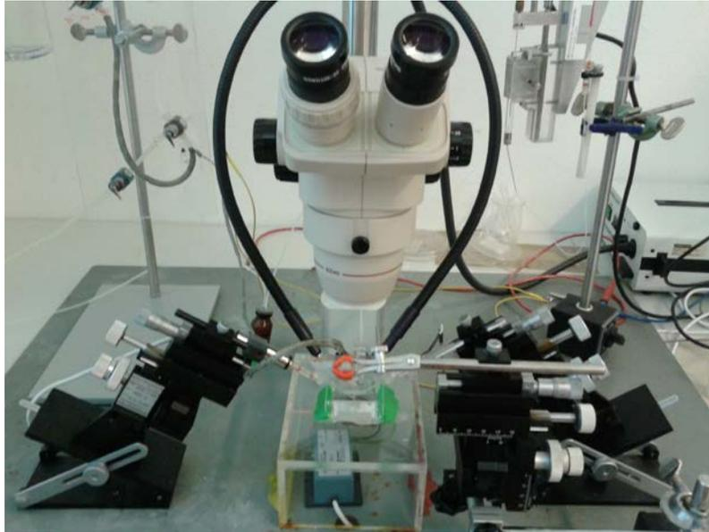
**Fig.7:** The picture shows our two-electrode voltage clamp setup. Cells are placed in a bath (between green mark) containing Xenopus Ringer solution below a stereomicroscope and get impaled with two measurement electrodes by using micromanipulators (black, on each side). Right on top of the cell is the applicator (orange) that is connected with a liquid suction system (self-made picture).
