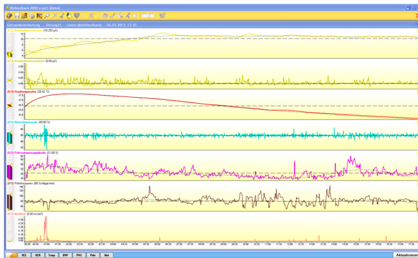
Figure 7: user interface of Biofeedback 2000 x-pert software with visualization of the parameters in lines (orange: SCL, yellow: SCR, red: finger temperature, blue: BVP, violet: PVA, brown: pulse, pink: motility)
