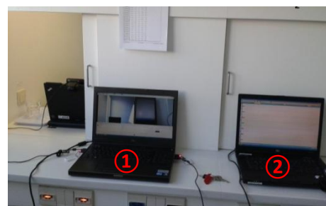
Figure 10: 1. laptop ( Dell precision ) with Media Recorder® software 2. laptop ( HP compaq ) with Biofeedback 2000 x-pert software and webcam Logitech C600
