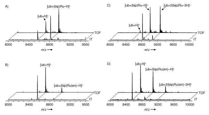
**Figure 2.** The deconvoluted mass spectra show the efficiency of adduct detection for the reaction of 1 and 2 with ubiquitin (ub) at different molar ratios after 48 h: A) 1 + ub (1:1), B) 2 + ub (1:1), C) 1 + ub (2:1) and D) 2 + ub (2:1). Identical samples were analyzed by ion trap (IT) and time-of-flight (ToF) electrospray (ESI) mass spectrometry.
