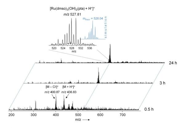
Figure S6. ESI-IT mass spectra of 1 in dimethylsulfoxide. The solution was diluted with water : methanol (1 : 1) prior to injection into the mass spectrometer.
