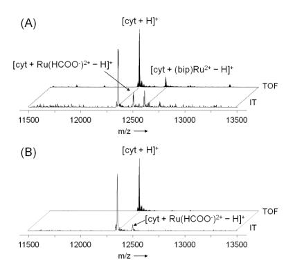
**Figure S1**. ESI-IT and ESI-TOF mass spectra of identical samples of **1** (A) or **2** (B) incubated with cytochrome C at a metal-to-protein ratio of 1:1 for 48 hours.
