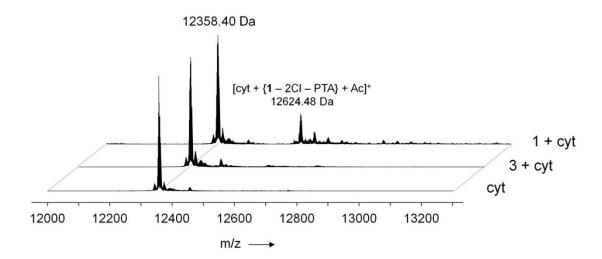
**Figure S3.** Deconvoluted mass spectra of cytochrome C and **1** or **3** after incubation for 24 h. The mixture was incubated at a 3 : 1 metal-to-protein ratio in buffer (pH 7.7).
