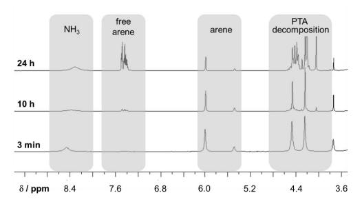
Figure S8. Time-dependent <sup>1</sup>H NMR study on the stability of 1 in dimethylsulfoxide- $d^{6}$ .
