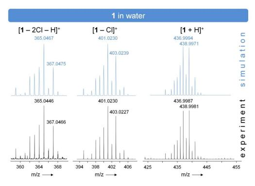
Figure S11. Experimental isotopic distributions and simulations of the mass signals of 1 in water.
