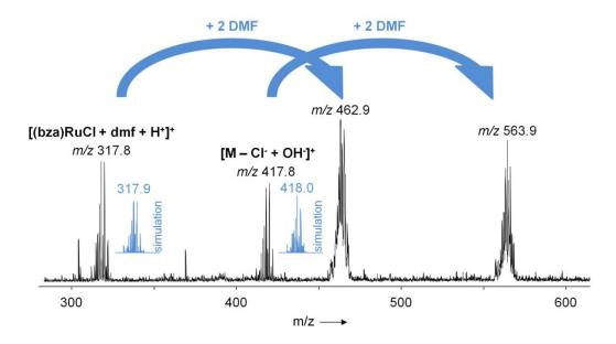
**Figure S9.** ESI-IT mass spectrum of **1** in dry dimethylformamide after 24 h. The solution was diluted with water : methanol (1 : 1) prior to injection into the mass spectrometer.
