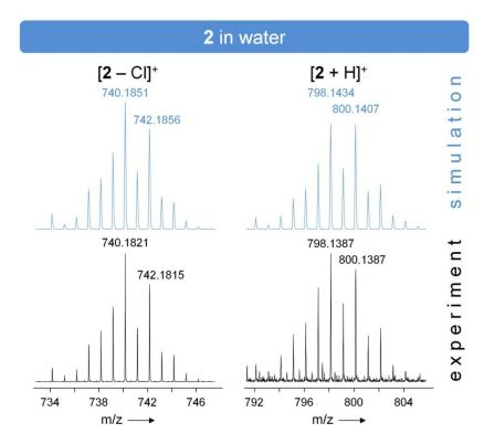
Figure S12. Experimental isotopic distributions and simulations of the mass signals of 2 in water.
