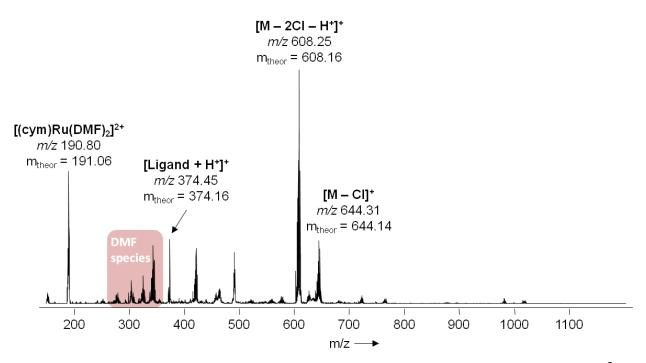
**Figure S5**. Full mass spectrum of **10** obtained by the reaction between  $[Ru(\eta^6-p-cymene)Cl_2]_2$  and 2 equivalents of **2**. Representative mass spectrum for reaction times 3-24 h. DMF species are Ru(cym) adducts with DMF, which was the solvent used for the reaction.
