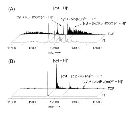
**Figure S2**. ESI-IT and ESI-TOF mass spectra of identical samples of **1** (A) or **2** (B) incubated with cytochrome C at a metal-to-protein ratio of 2:1 for 48 hours.
