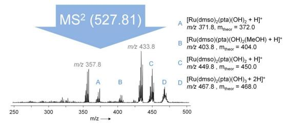
Figure S7. ESI-IT tandem mass spectrometric analysis of the signal at m/z 527.81 from the solution of 1 in dimethylsulfoxide after 24 h.
