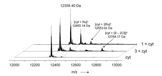
**Figure S5.** Deconvoluted mass spectra cytochrome C and **1** or **3** after incubation for 48 h. The mixture was incubated at a 3 : 1 metal-to-protein ratio in water (pH 6.0).
