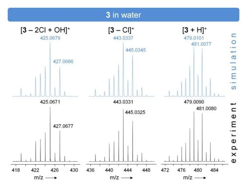
Figure S13. Experimental isotopic distributions and simulations of the mass signals of 3 in water.
