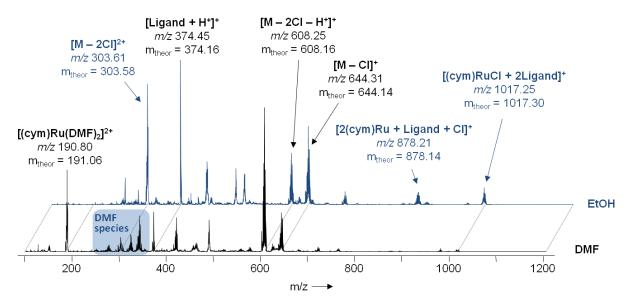
**Figure 2**. Full ESI-IT mass spectra of the reaction mixture yielding compound **10** after 3 h. The reactions were carried out in dimethylformamide (DMF) and ethanol (EtOH). The reaction using DMF as a solvent leads to a more selective formation of **10**.
