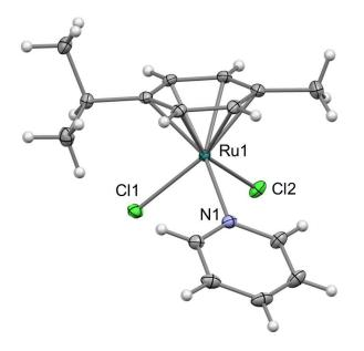
**Figure 3.** Molecular structure of the neutral complex  $[(\eta^6-p\text{-}cymene)Ru(pyridine)Cl_2]$  **6**. Selected bond lengths [Å] and angles [°]: Ru1-C(1–6)<sub>av</sub> 2.186, Ru1-N1 2.1368(12), Ru1-Cl1 2.4194(4), Ru1-Cl2 2.4026(4); N1-Ru1-Cl1 85.94(3), N1-Ru1-Cl2 86.81(4), Cl1-Ru1-Cl2 87.328(14).
