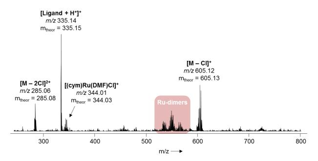
**Figure S1**. Full mass spectrum of **7** obtained by the reaction between  $[Ru(\eta^6-p-cymene)Cl_2]_2$  and 2 equivalents of **3**. Representative mass spectrum for reaction times 3-6 h. Ru-dimers denote dimeric hydrolysis products resulting from chloride and biotin ligand release.
