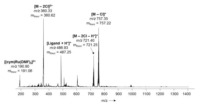
**Figure S6**. Full mass spectrum of **11** obtained by the reaction between  $[Ru(\eta^6-p-cymene)Cl_2]_2$  and 2 equivalents of **4**. Representative mass spectrum for reaction times 3-24 h.
