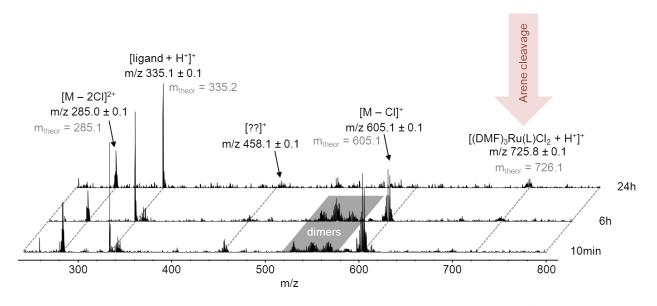
**Figure S2**. Mass spectrum of **7** obtained by the reaction between  $[Ru(\eta^6-p-cymene)Cl_2]_2$  and 2 equivalents of **3**. Representative mass spectrum for reaction times of 10 min, 6 and 24 h. Substantial arene cleavage was observed after more than 6 h of incubation.
