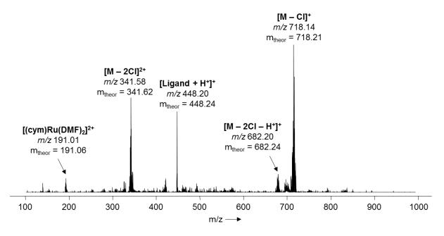
**Figure S4**. Full mass spectrum of **8** obtained by the reaction between  $[Ru(\eta^6-p-cymene)Cl_2]_2$  and 2 equivalents of **5**. Representative mass spectrum for reaction times 3-24 h.
