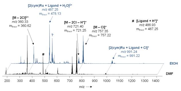
**Figure S7**. ESI-IT mass spectra of the reaction mixture yielding compound **11** after 3 h. The reactions were carried out in dimethylformamide (DMF) and ethanol (EtOH). The reaction using DMF as a solvent leads to a more selective formation of **11**.
