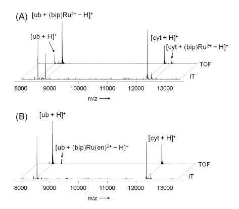
**Figure S3**. ESI-IT and ESI-TOF mass spectra of identical samples of **1** (A) or **2** (B) incubated with a mixture of ubiquitin and cytochrome C at a metal-to-protein ratio of 1:1:1 for 48 hours.
