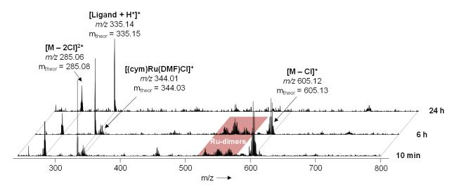
**Figure S3**. Full mass spectra of the reaction products obtained by the reaction between  $[Ru(\eta^6-p\text{-cymene})Cl_2]_2$  and 2 equivalents of **3**, after 10 min, 3 h and 24 h. Ru-dimers denote dimeric hydrolysis products resulting from chloride and biotin ligand release.
