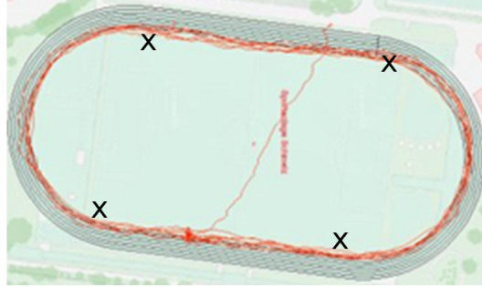
Figure 5.2: GPS processing of the running scenario. The lane of the athletic track was adjusted with the knowledge of its geometrical model and the 4 GPS coordinates (X).
