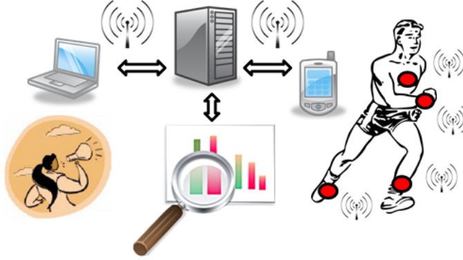
Figure 1.3: The desired structure of an MC system for runners. The smart-phone of the runner should gather data from the sensors (red points) via a BSN. The preprocessed data will be sent to a server via the Internet and stored in a database. The analysis of the actual training should be carried out by experts e.g., sport scientists or biomechanists, or server-side routines. Finally, the runners should be supported by feedback.
