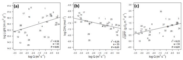
**Figure 11** Discharge (Q) affects (a) light, (b) dissolved inorganic nitrogen (DIN) and (c) gross primary production (GPP). Solid lines are the statistically significant linear regressions Site code is given in Table 3.
