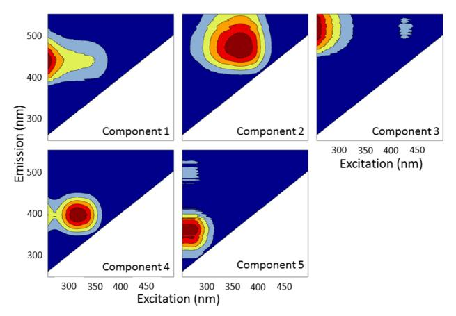
Figure 4 Excitation and emission matrices (EEMs) of the five components modelled with the PARAFAC analysis.
