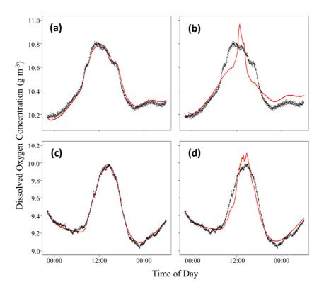
**Figure 7** Black points indicate measured DO concentrations and the red line indicates predicted DO concentrations by the one-station model for site 2 (**a**,**b**) and site 15 (**c**,**d**) with saturating photosynthesis-irradiance curve (**a**,**c**) and with linear photosynthesis-irradiance relationship (**b**,**d**).
