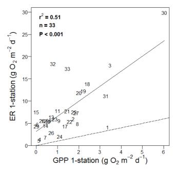
**Figure 9** Relationship between daily ecosystem respiration at in-situ temperature (ER) and daily gross primary production (GPP) estimated by the one-station approach. Solid line is the statistically significant (P < 0.001) linear regression ( $ER = 3.2 (\pm 1.1) + 3.4 (\pm 0.6) \times GPP$ ). Dashed line indicates 1:1 relationship. Site code is given in Table 3.
