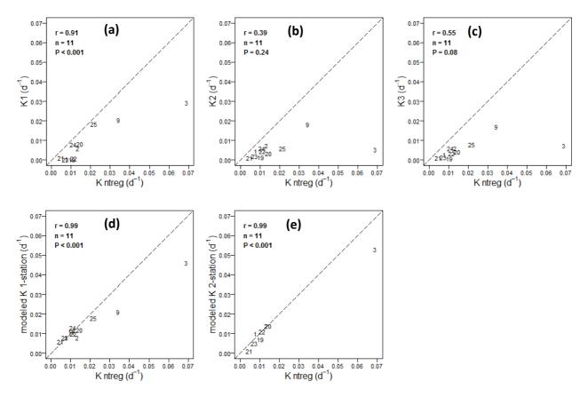
**Figure 6** Correlations between reaeration coefficients derived by night-time regression (K ntreg) and reaeration coefficients derived by empirical equations (11) to (13) (**a-c**) and modeled reaeration coefficients by one-station (**d**) and two-station (**e**) approach. Dashed lines indicate 1:1 relationships. Site code is given in Table 3
