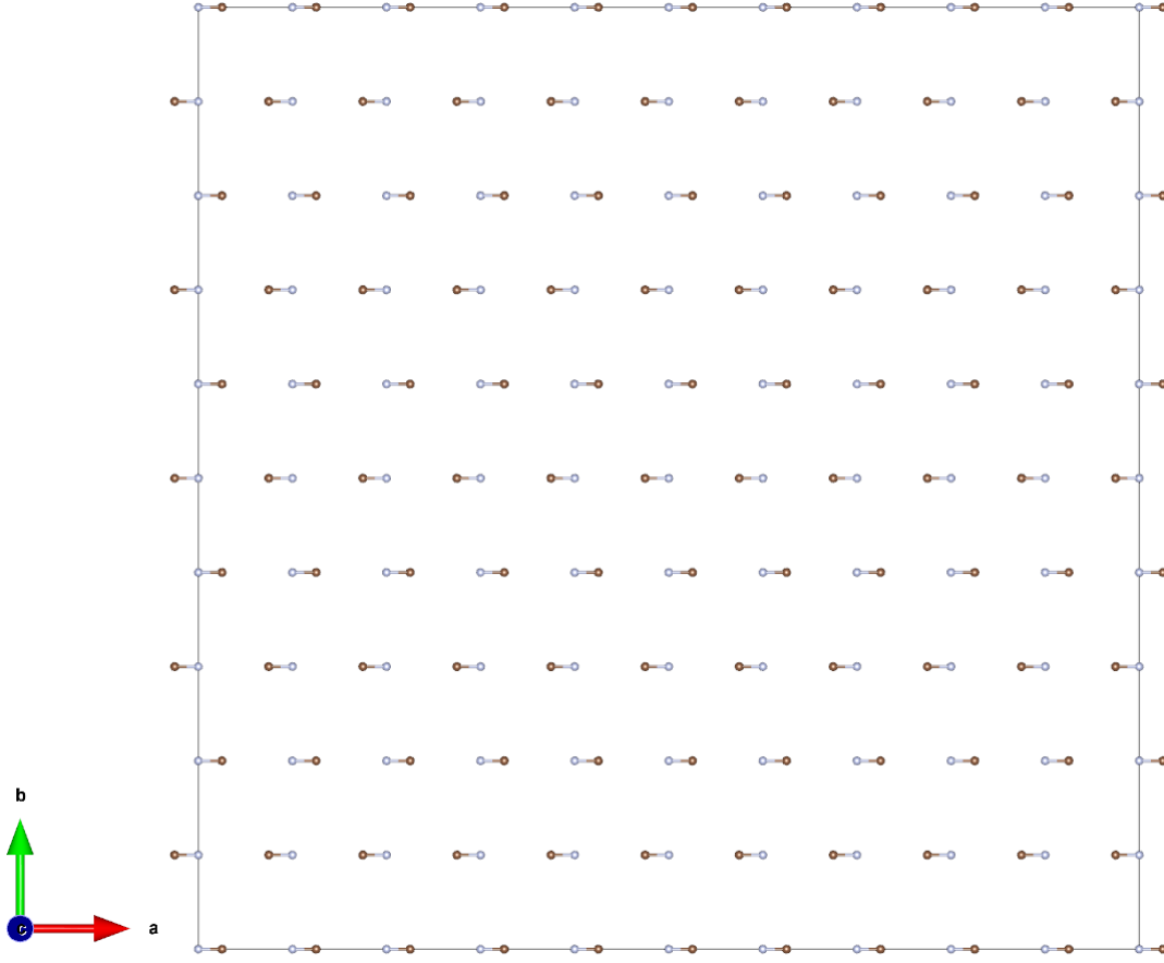
Figure 5.41: Single 10 \times 10 \times 1 dipole layer at 0K
