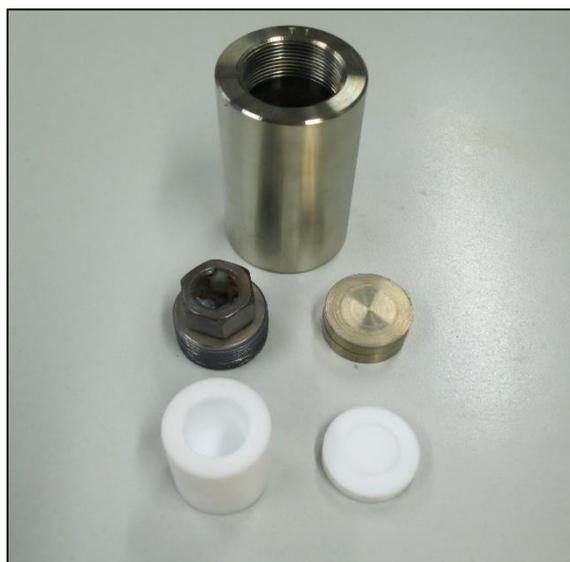
Figure 2. Morey-autoclave with Teflon vessel.
