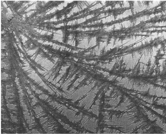
**Figure 3.3:** Electron micrograph of a thin  $\alpha$ -iPP film, exhibiting lamellar branching at angles of  $80^\circ$  to  $100^\circ$  [38].
