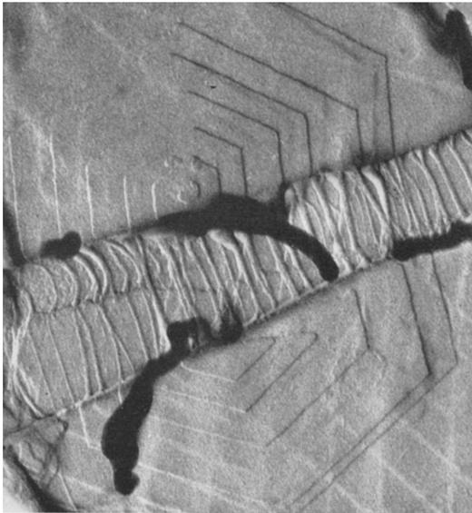
**Figure 3.8:** Microfibrils pulled out at the crack of polyoxymethylene (POM) single crystals [64]
