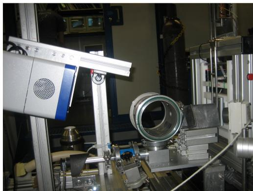
**Figure 4.6:** Two dimensional Pilatus detector
