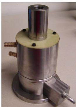
**Figure 4.1:** Compression chamber used for the production of  $\gamma$ -samples
