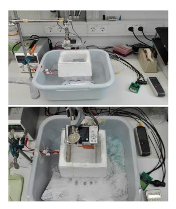
Figure 7.2.2. Photo-graphic pictures of the cooling-device used for the droplet-freezing assay
