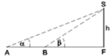
$$AB = 100\text{m}, \alpha = 15,8^\circ, \beta = 38,1^\circ$$
