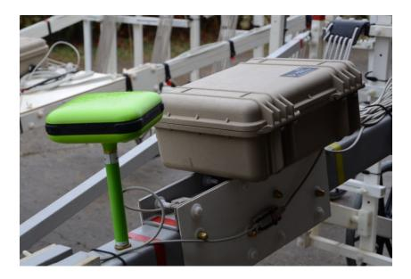
Figure 53: GNSS receiver (rover) mounted in front of the Peli case, which holds the datalogger (© M.Kucera).
