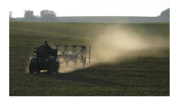
Figure 54: Motorized magnetometers are operated at an average speed of 15 to 25 km/h (© M.Kucera).
