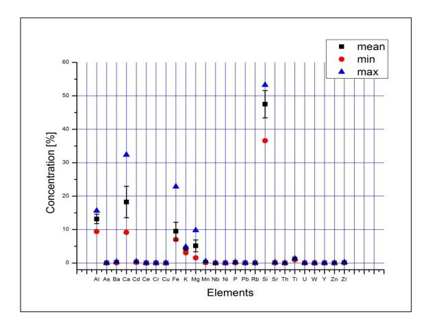
Figure 23: Variability of all measured elements with range and error bars from Hornsburg 1, Ditch 1. The scale is optimized for the display of Al, Ca, Fe, K, Mg and Si.
