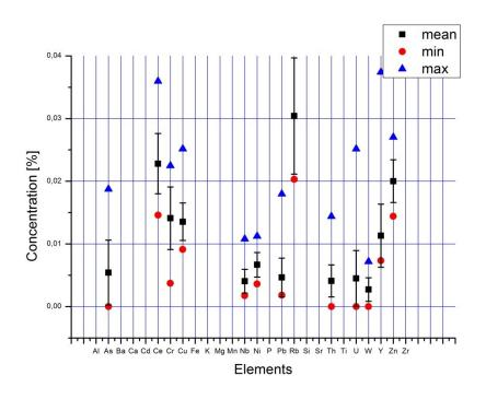
Figure 29: Variability of trace elements with range and error bars from Hornsburg 1, Ditch 1. The scale is optimized for the display of As,, Ce, Cr, Cu, Nb, Ni, Pb, Rb, Th, U, W, Y and Zn.
