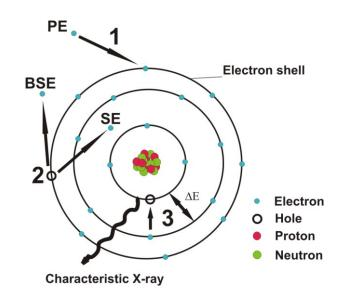
Figure 4: Schematic atomic model; Characteristic X-ray emission (©Kucera).
