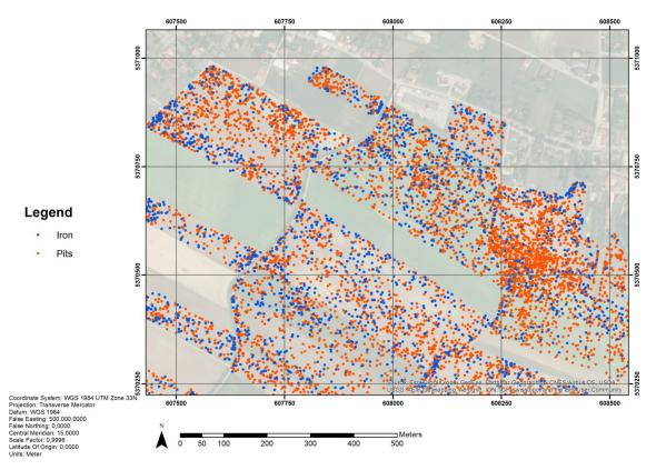
Figure 58: Distribution of magnetic anomalies caused by iron objects and archaeological features (pits). The location of iron often indicates old pathways (© LBI ArchPro, M.Kucera).
