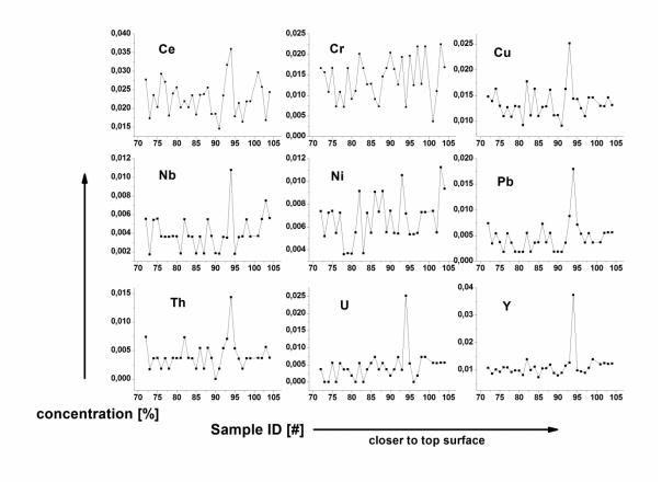
Figure 31: Comparison of minor elements. The scale of y-axis is optimized for every elemental distribution. The spatial development of Cu was used to classify SU.
