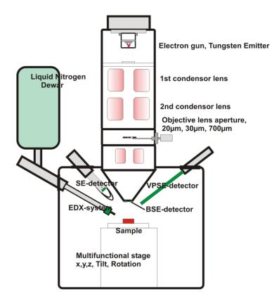
Figure 3: The main components and detectors of a VP-SEM with an EDX-system (Leo EVO 60plus, Zeiss)(©M.Kucera).
