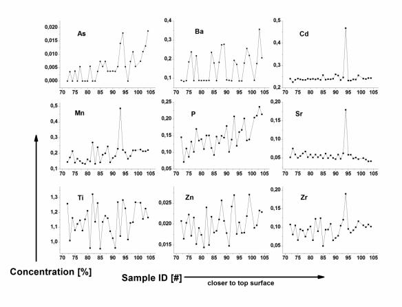
Figure 30: Comparison of minor elements. The scale of y-axis is optimized for every elemental distribution. The spatial development of Mn was used to classify SU. Mind also to compare P and Zn.
