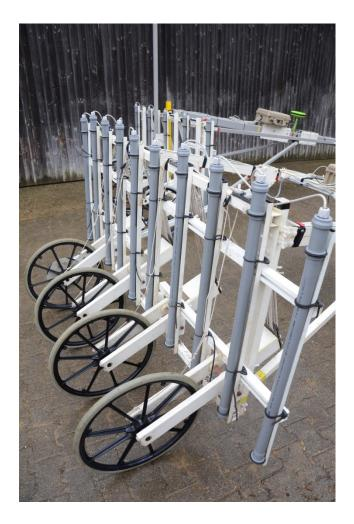
Figure 52: 10 Foerster FEREX CON650 gradiometer probes mounted on the cart. The wheels are independently suspended (© M.Kucera).
