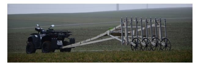
Figure 51: Motorized magnetic prospection. The multi-sensor array is towed by an ATV (© M.Kucera).
