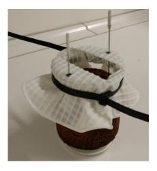
Figure 4. Electrodes fixed by a silicon mesh
