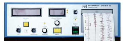
Figure 6: Thymatron® System IV. The device records parameters like EEG as well as EMG and delivers the energy for the electrical stimulation through electrodes. Figure by SOMATICS, LLC (SOMATICS LLC, Retrieved 21.03.2018)
