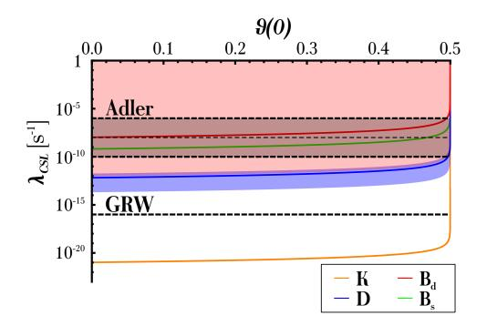
Figure 5.1: These plots show the values of  $\vartheta(0)$  versus the deduced collapse rate based on the input parameters  $\Gamma_{H}^{\exp}$ ,  $\Gamma_{L}^{\exp}$ ,  $\Delta m^{\exp}$  for the different types of neutral mesons (including experimental errors highlighted by the shaded areas). As a reference mass the respective rest mass of the neutral mesons is assumed.
