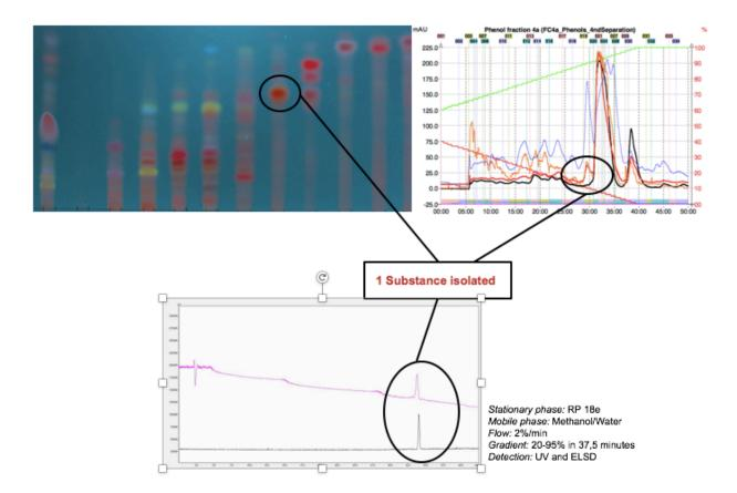
**Figure 16:** TLC of combined fractions (1-11) of 03b, 04a and 04b (above left), FC04a of Phenols (above right) and HPLC of fraction 7 (below); the circles indicate the pure compound respectively
