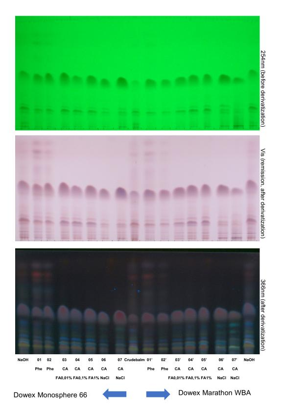
Figure 10: TLC comparison of Dowex Monosphere 66 and Dowex Marathon WBA
