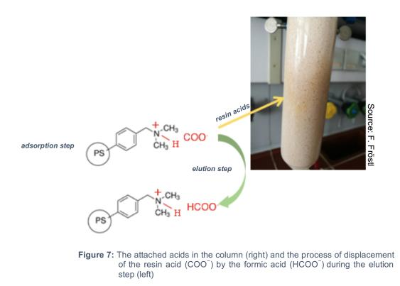
In this so-called **adsorption step** acids are retained in the column while other substances, like phenols, alcohols and apolar compounds, can elute. The column is flushed with a 90 % MeOH solution. As a result, everything that does not bind to the ion exchange resin is washed off and accumulates in the first fraction, the so-called phenol fraction.
