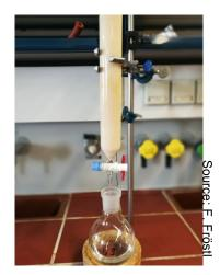
**Figure 5:** Dowex Marathon WBA, during the exchange of ions
