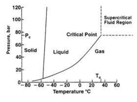
Figure 6: Phase diagram for carbon dioxide
