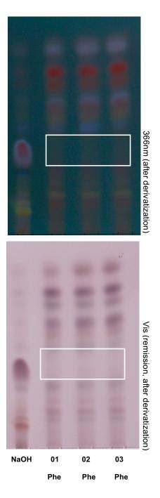
**Figure 14:** TLC comparison, showing the depletion of resin acids in the phenol fractions (marked area)
