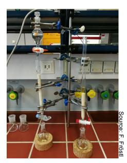
Figure 8: Dowex Monosphere 66 (left), Dowex Marathon WBA (right)
