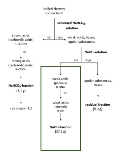
Figure 4: Liquid-liquid extraction steps made by Göls T. (Langeder, 2017)
