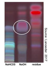
**Figure 3:** TLC-fingerprint comparison of NaHCO<sub>3</sub>-fraction, Residue-fraction and NaOH-fractions (high accumulation of diterpenes is market)
