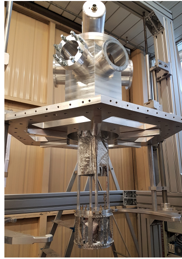
(b) Cold head, cooling line and target cell wrapped in super-insulation.
