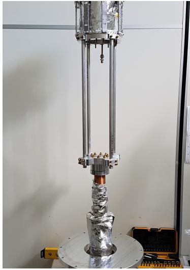
(a) Cooling structure for the target cell before installation at the setup.
