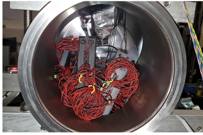
(a) Detector units placed inside the vacuum chamber to check for outgassing and to determine the highest achievable vacuum.
