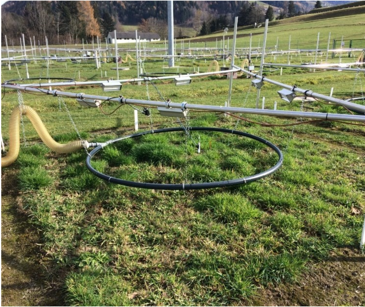
Figure 2 | Experimental setup: a miniFACE ring for CO 2 fumigation and infrared heaters fixed on a triangular frame to manipulate air temperature.
