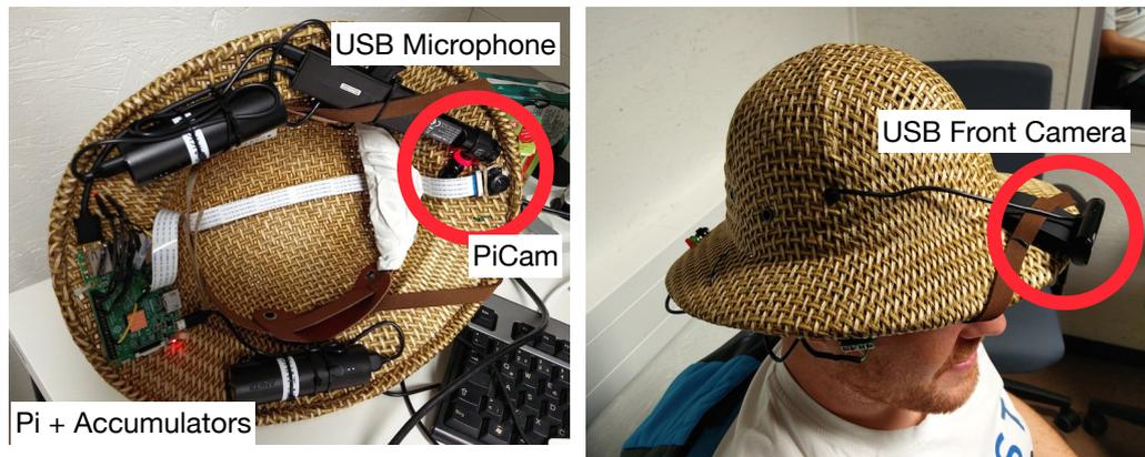
Figure 4.14: The CoCoHAT with its different components: The core is a Raspberry Pi plus two accumulators. A PiCam films the user's interaction on the smartphone (see left). A USB microphone and a USB front camera record the surroundings (see right).
