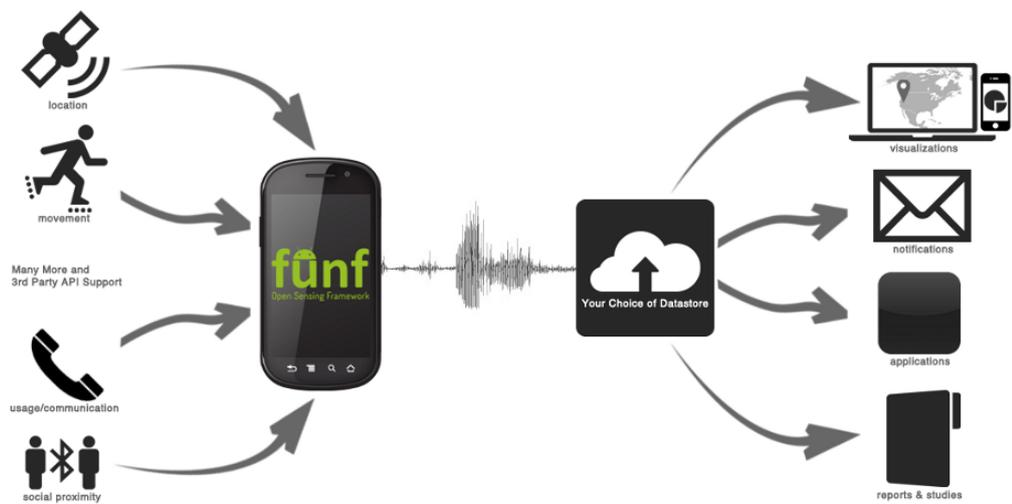
Figure 4.4: Input and output capabilities of the Funf framework (Source: Funf website)
