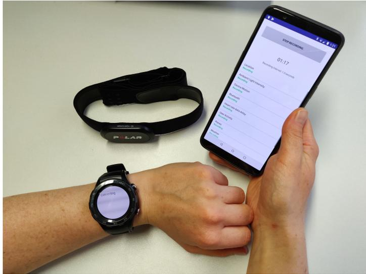
Figure 4.10: Recording screen of CoConUT, together with a chest belt and a smartwatch
