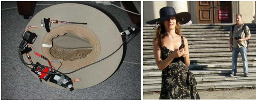
Figure 4.1: The LiLiPUT prototype, which is a “wearable lab environment” for user tests in the form of a hat [Rei+07]
