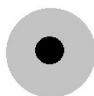
Figure 4: Simple graphic of a concentric spherical core-shell nanoparticle, consisting of a simple inner core and a shell of a different material.
