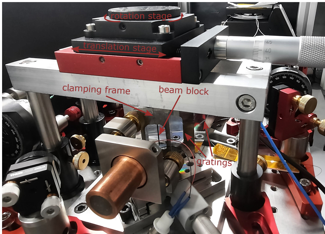
Figure 2.2 – The tunable mechanical spectral filter was implemented by clamping a thin aluminum beam block foil (Thorlabs BKF12 foil) in an aluminum frame. The frame was attached to a rotation stage, which in turn was mounted on a translation stage.
