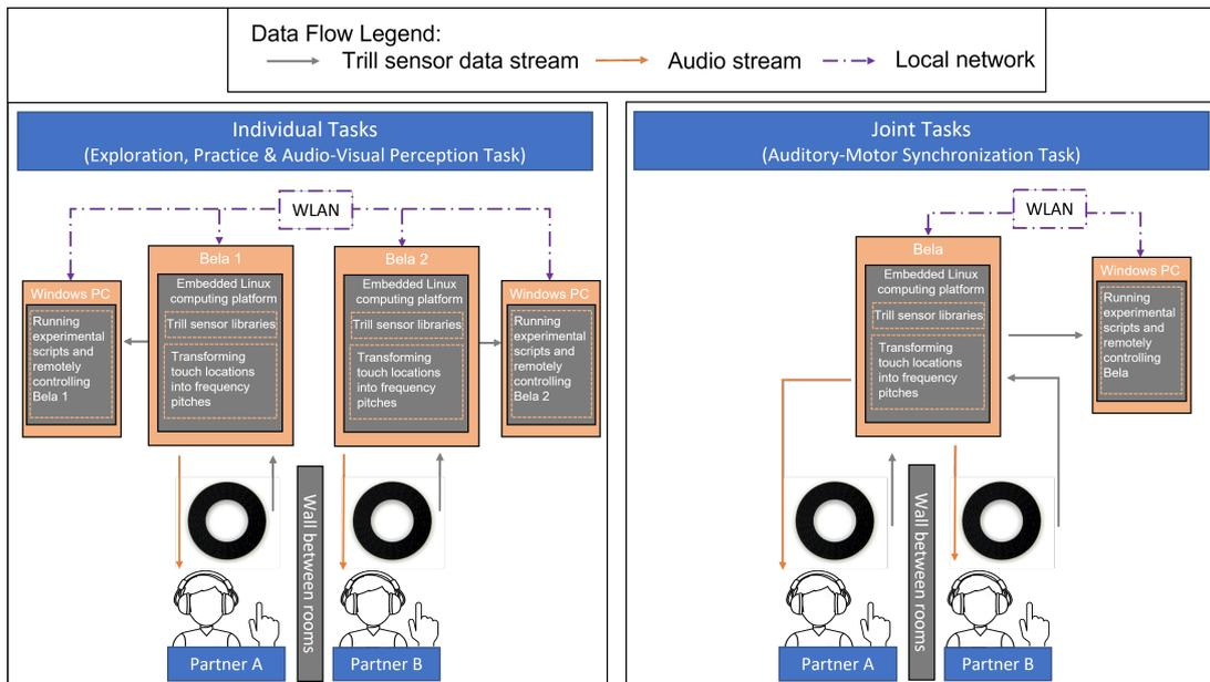
**Figure 2.4.:** The experimental set-up. (a) shows the general set-up of the rooms and the connection cables. Orange arrows indicate audio cables, blue arrows show connection cables for the Trill sensors, (b) displays one partner's testing room with headphones, camera and a touch sensor, (c) shows the data flow in the experiment.
