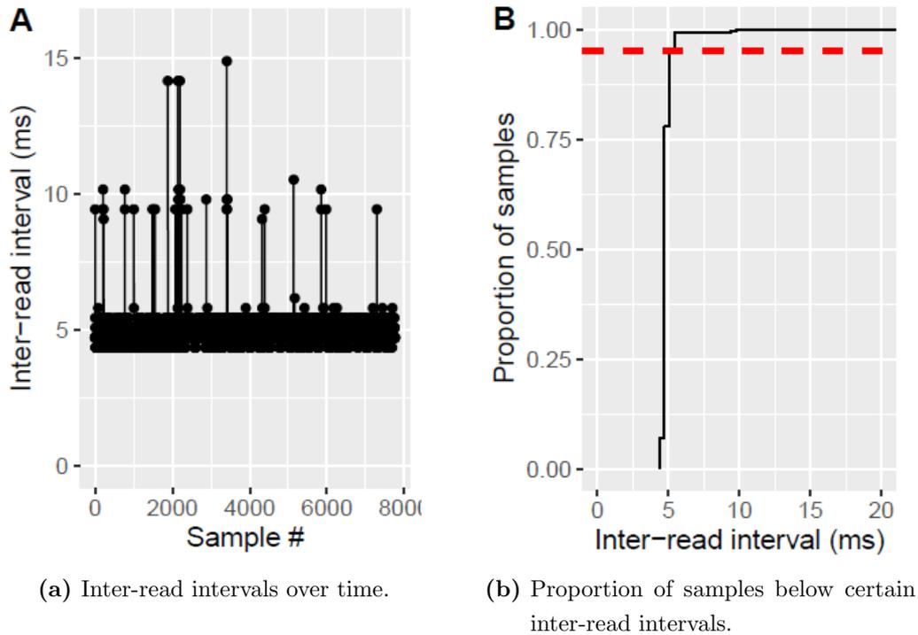
**Figure 2.3.:** The inter-read intervals of new touch locations which are mostly 5 ms. Subfigure (a) shows the inter-read intervals in ms on the y-axis with values at around 5 ms. The x-axis shows the number of samples. (b) reports on the proportion of samples (y-axis) below certain inter-read intervals (x-axis). One can clearly see that most samples are extracted every 5 ms.
