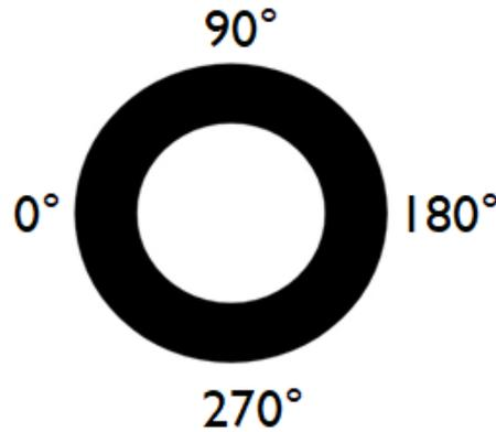
**Figure 2.5.:** The Trill sensor with the labelling convention used. The 0° point was to the left, 90° at the top, 180° to the right and 270° at the bottom of the ring-shaped sensor.
