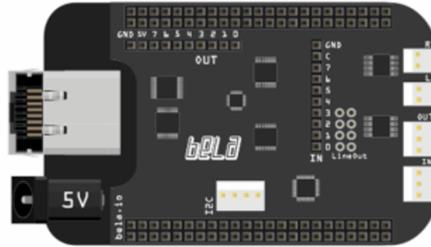
**Figure 2.2.:** The embedded computing platform Bela used for the experiment (taken from (BelaPlatform, 2021b)).
