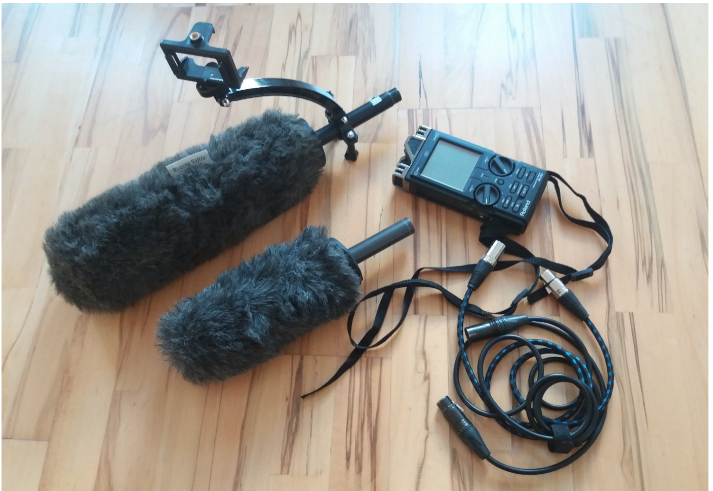
Figure 6: Picture of both microphones, the recorder, and the repurposed bicycle camera mount.
