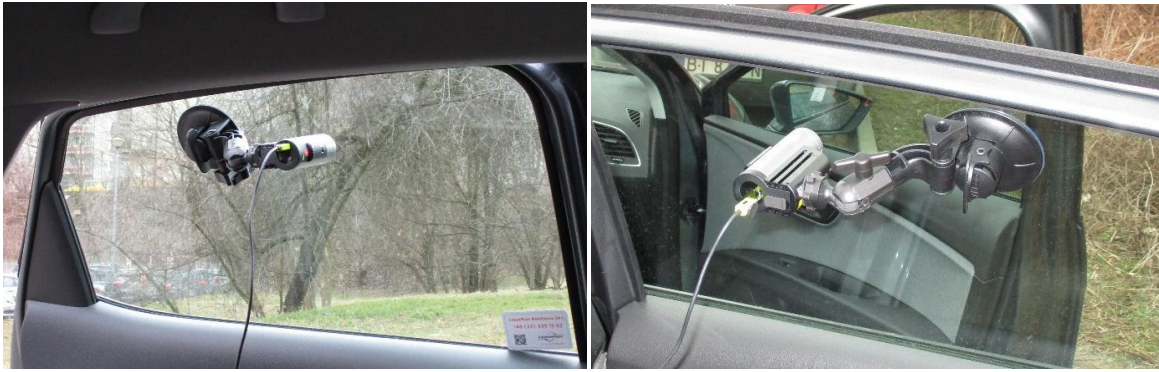
Figure 6: Cameras mounted on left and right backseat windows; Source: Prof. Dr. Michael Leitner
