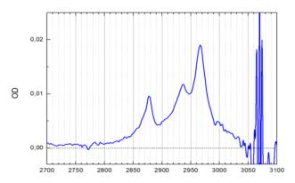
Figure 16: MIR spectrum of water independent bands assigned to the TBA cation.
